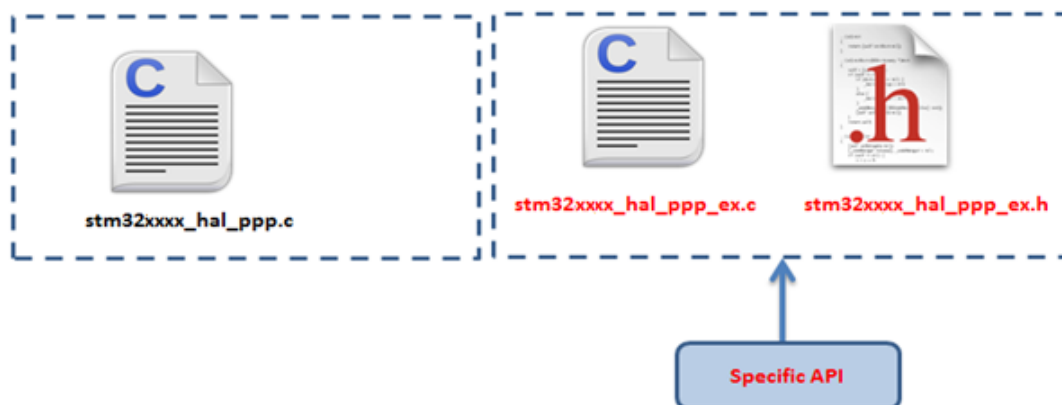
Figure 2. Adding device-specific functions
